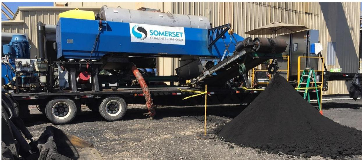
**Figure 2. Onsite Testing with Sub325™ Centrifuge**
